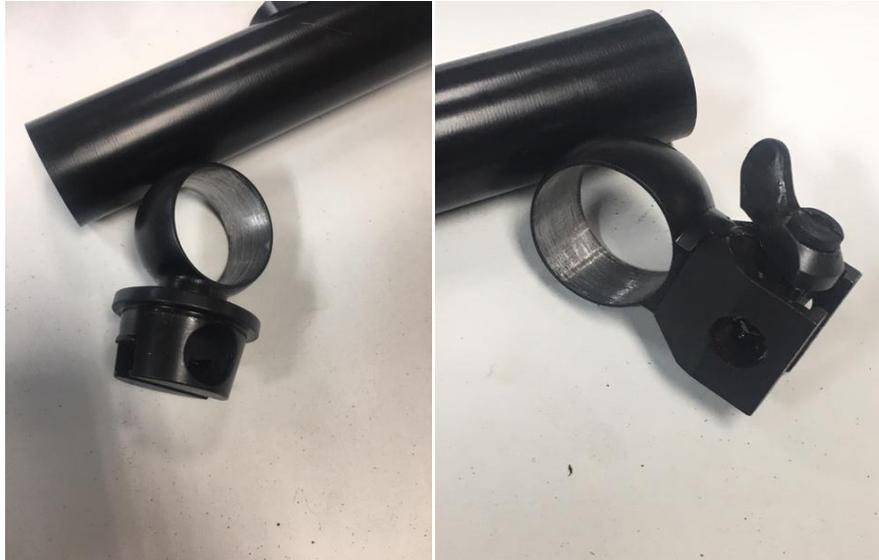
Once done correctly, the ring should slide over the main tube with the minimum of clearance between the ring and the main tube. This is important in the next step which is affixing the ring to the main tube.
