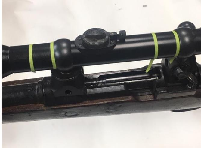
7. Using sand paper or emery cloth completely remove any coating between the marks (the area that will be covered by the rings)
