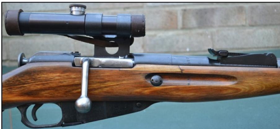
The mount assembly does allow for course elevation adjustment, the front of the saddle pivots on a ball joint, which by adjusting two small screws can provide course elevation and depression. There is no scale, so any adjusted movement is course and approximate. Slackening of the large thumb screw permits the whole mount and scope to be removed, thus preventing damage during transit.
